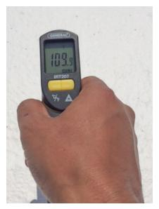
The energy saving benefit associated with a "cool roof" installation is very significant. The highly solar reflective finish material have been proven to lower surface temperatures by up to 65°F, resulting in air-conditioning energy savings as high as 40% when installed over dark surfaces.
